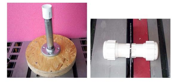
Now you have to modify the slip joint. The slip joint holds the extending pole, but it must attach to the PVC adapter. Here you get a 2-for-1 ... we saw the slip joint in half. Use the 1-1/2" PVC coupler to join the PVC pipe adapter and the slip ring using PVC pipe glue. I like to insert the extending pole in the assembly as it dries to hold the proper alignment.
