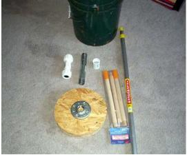
The first step is to measure the inside bottom of your bucket. Surprise, surprise, they are not all the same! Then cut a few circles out of the chipboard and glue them together to make a steady base. I use my router with a circle cutting guide to make nice circles.
