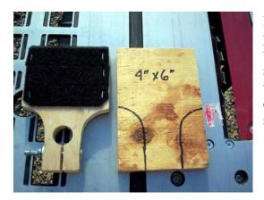
I then cut out the ammo holders to grip the top portion of the extendable pole. I use a 3/16 bolt and wing-nut to clamp the holder in place. I've also stapled Velcro to the top of the pictured holder and then can place the other side of the tape to a pellet tin or pellet holder to keep it from falling off during slight bumps.
