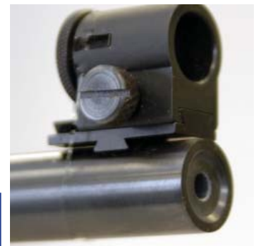
The tunnel front sight on the Savage Mark I comes with six interchangeable apertures and four post inserts.
