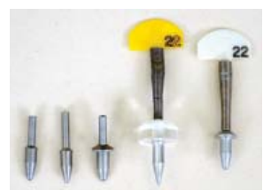
.22 cal. rifle and pistol gauges, l. to r., ISSF/USAS Inward, NRA Inward, A-36 Inward, NRA Inward, A-36 Inward. The first three gauges are manufactured by Gunsmithing, Inc.; the other two by RIG.
