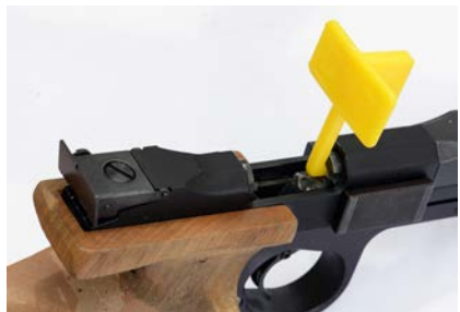
Cleared semi-auto pistol with slide back, magazine removed, chamber empty and safety flag inserted.
