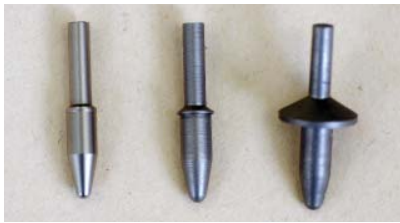
10-Meter air rifle and pistol scoring gauges, l. to r., Air Rifle/Pistol Inward, Air Rifle Outward and Air Pistol Outward. Note the small flange on the inward gauge and the larger flanges on the outward gauges. The gauges shown here are all Gunsmithing, Inc. gauges.
