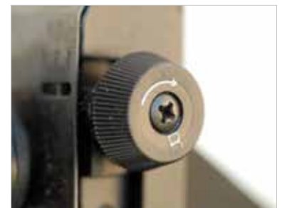
Sights sold with rifles marketed by USA companies have arrows indicating the direction the shot/shot group will move when turned in that direction. Be sure to look carefully at the sight knobs, however, because some USA sights turn in the opposite direction from other USA sights.
