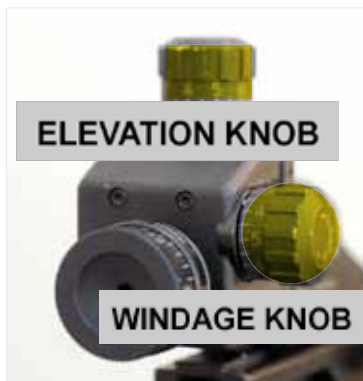
New shooters need to understand how the elevation (top) and windage (right) knobs on their rear sights work.
