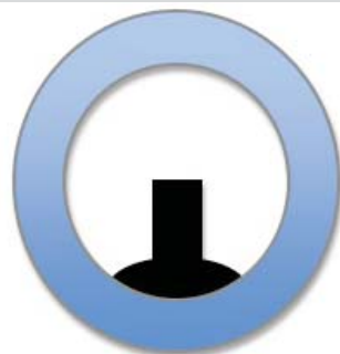
Sight alignment with a post front sight.
