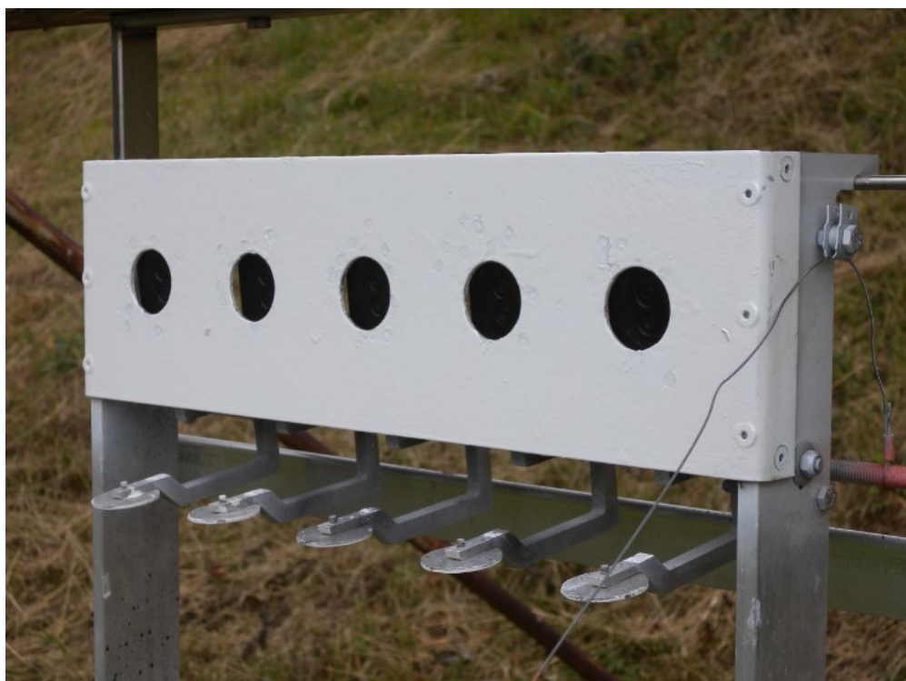
Target Sprint competitors shoot 5-shot series standing on knock-down targets. When a shot hits the target, the paddle rises to cover the target.
