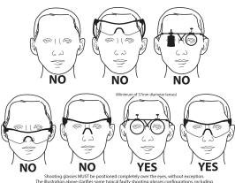
Shooting glasses MUS1 be positioned compiletely over the eyes, without exception. The illustration above clarifies some typical faulty shooting glasses configurations, including removing lenses, along with the proper sale orientation (bottom right). Lenses suspended from frames, covering the eyes, with a minimum diameter of 37mm are permissable.
