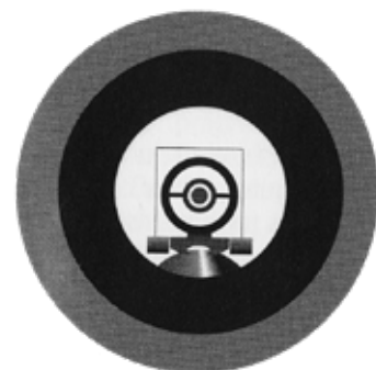
Sight picture includes the rear aperture, front sight, front sight ring and aiming bull on the target.
