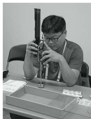
Proper trigger weighing technique is shown in this photo. Both elbows must be on the table as the pistol is lifted with the 500 g weight.
