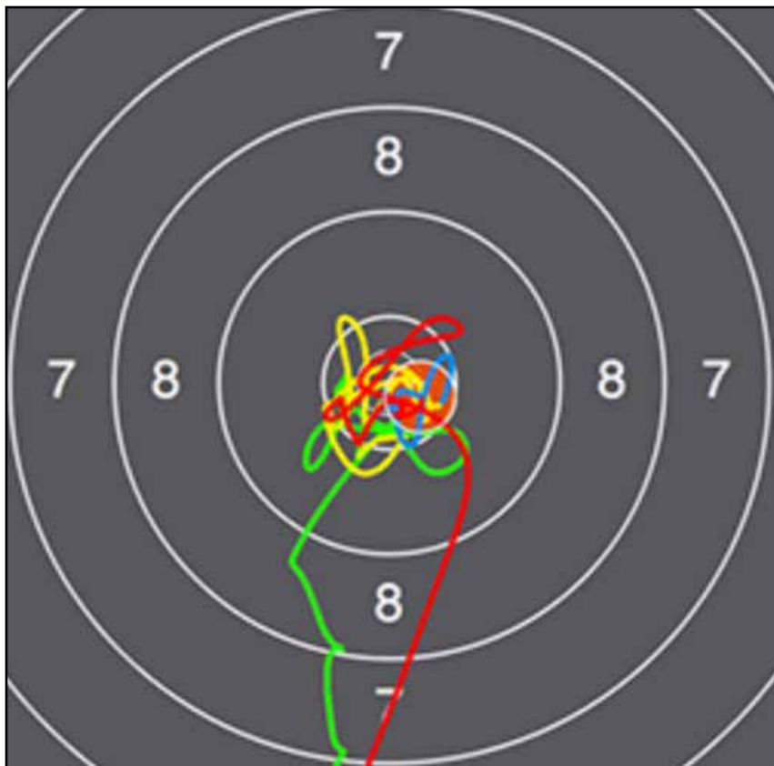
A SCATT training system display for one shot. The color changes show hold movements before (green), just before (yellow) and after (red) the shot.
