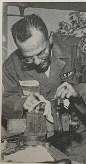
Weapons repair Sgt. R. Kraft, USA, works on an M1911 cal. .45 Service pistol. Weapons repair vans were available behind the firing lines for those using Service arms
