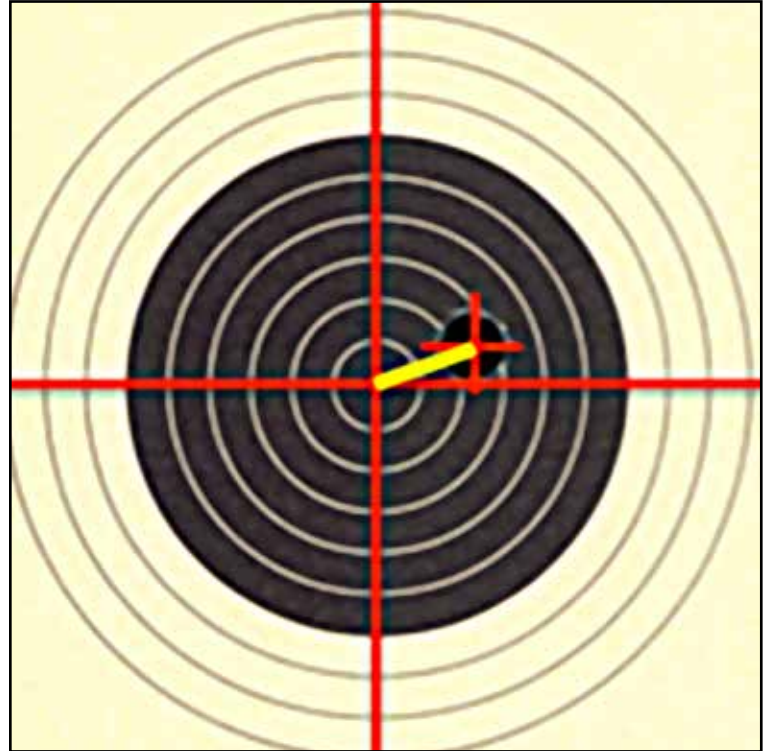
Orion scores shots by using optical scan images to measure the precise distance from the center of the aiming black (target) to the center of the shot hole.
