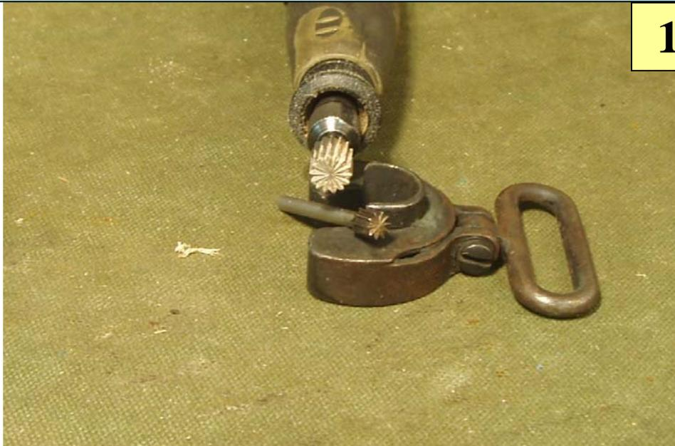
Try to remove only a little at a time and as evenly as possible. Remove only enough to level out the trigger group's fit.
