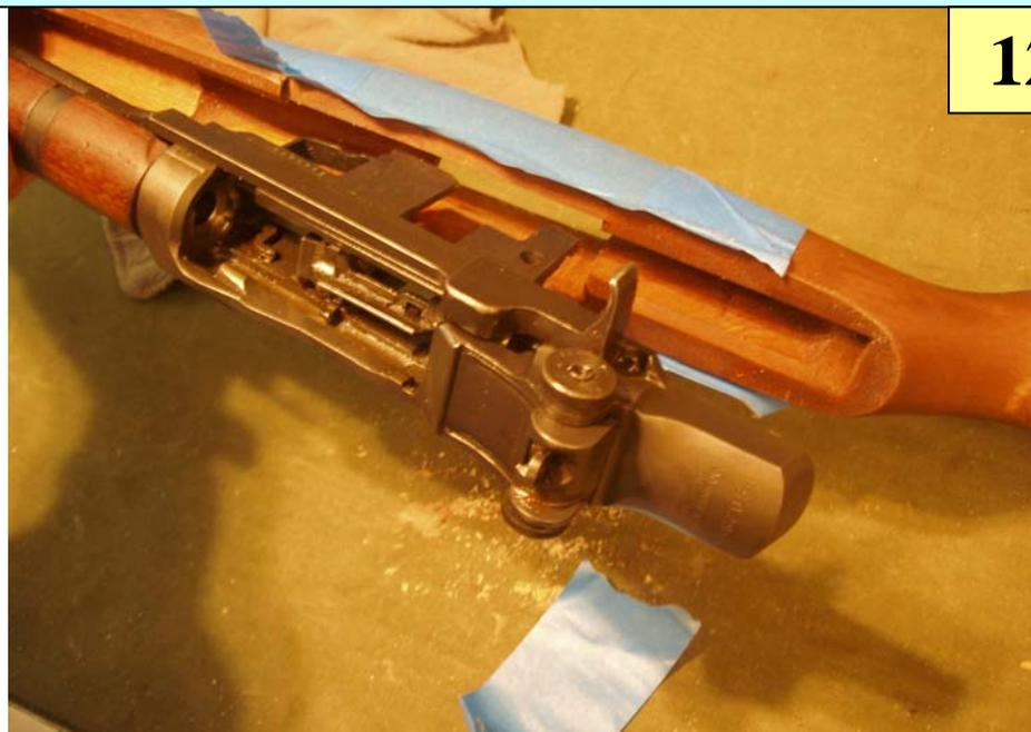
Measure your progress by the movement of the trigger guard toward locking up with the tightness you find acceptable. Make sure that you go slow and verify that the trigger group is fitting the stocks four contact surfaces evenly without gaps as shown in photo #3.
