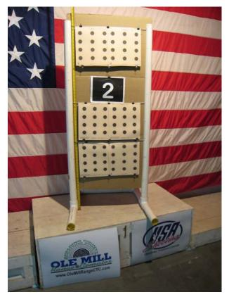
pressure caps in the front legs to dress the project up a bit. The yellow pressure caps really don't have a function other than esthetics. I added 4 sheet rock screws to the leg bottoms, outer edges, for leveling. This feature is seldom used but it's there if we need it.
