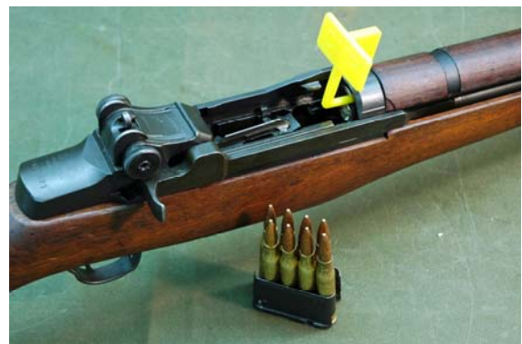
M1 Garand with ECI inserted ECIs must be in all firearms, at all times, except during preparation and firing periods.
