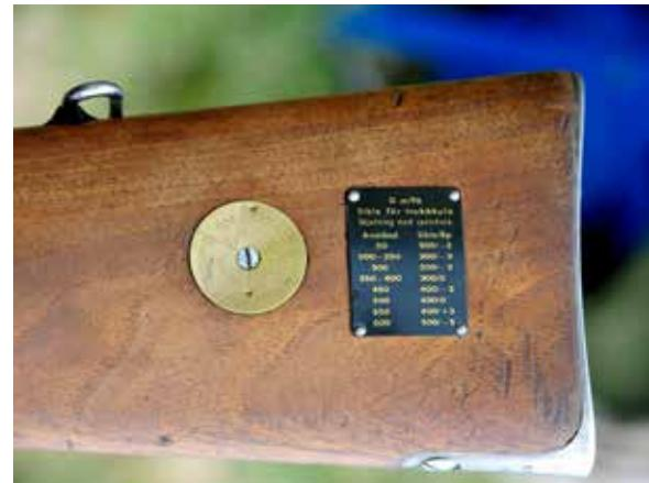
This close-up of a rifle buttstock shows affixed plates which provide as-issued information including caliber, bore condition and ballistics for the 6.5mm G/m96 Swedish Mauser rifle.
